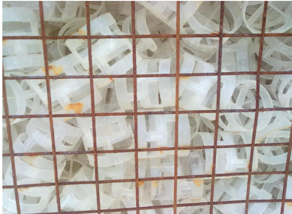
Steel cage with pall ring packing media
